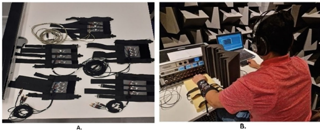
Fig. 8.2 (a) The apparatus used in Yeganeh et al. [59, 60]. The figure shows sleeves of stretchable material of five different sizes with different distances between actuators. (b) The experimental setup in Yeganeh et al. [59, 60]
