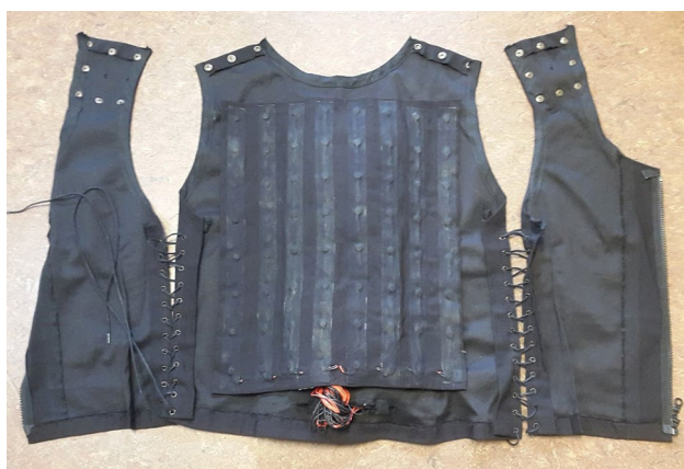
Fig. 1 The tactile vest with a 40-mm inter-tactor spacing (used in experiments 1–4)
